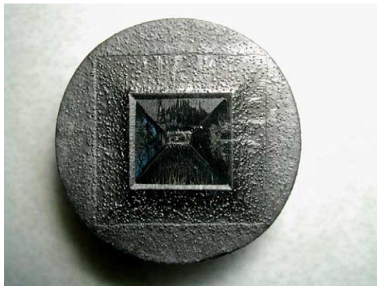
Fig. 2. Melt textured Y123 single crystal (22 mm diameter, 8 mm thickness) showing interfaces caused by termination/continuation of solidification at different undercooling temperatures.
